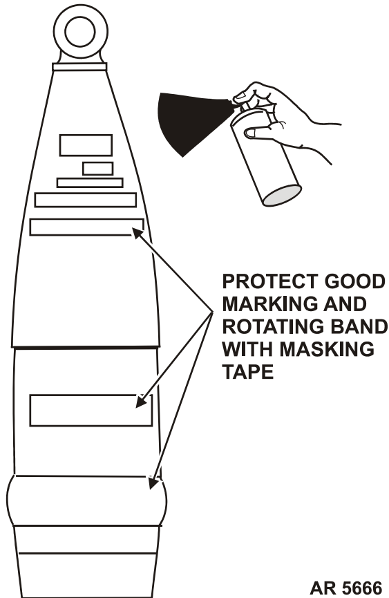
Figure 3-20. Using Spray Paint for Touchup.
